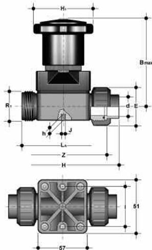
DIAPHRAGM VALVE COMPACT with unionised metric series plain female ends for solvent welding
