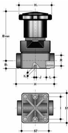
DIAPHRAGM VALVE COMPACT with BS parallel threaded female ends
