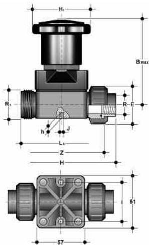
DIAPHRAGM VALVE COMPACT with unionised BS parallel threaded female ends
